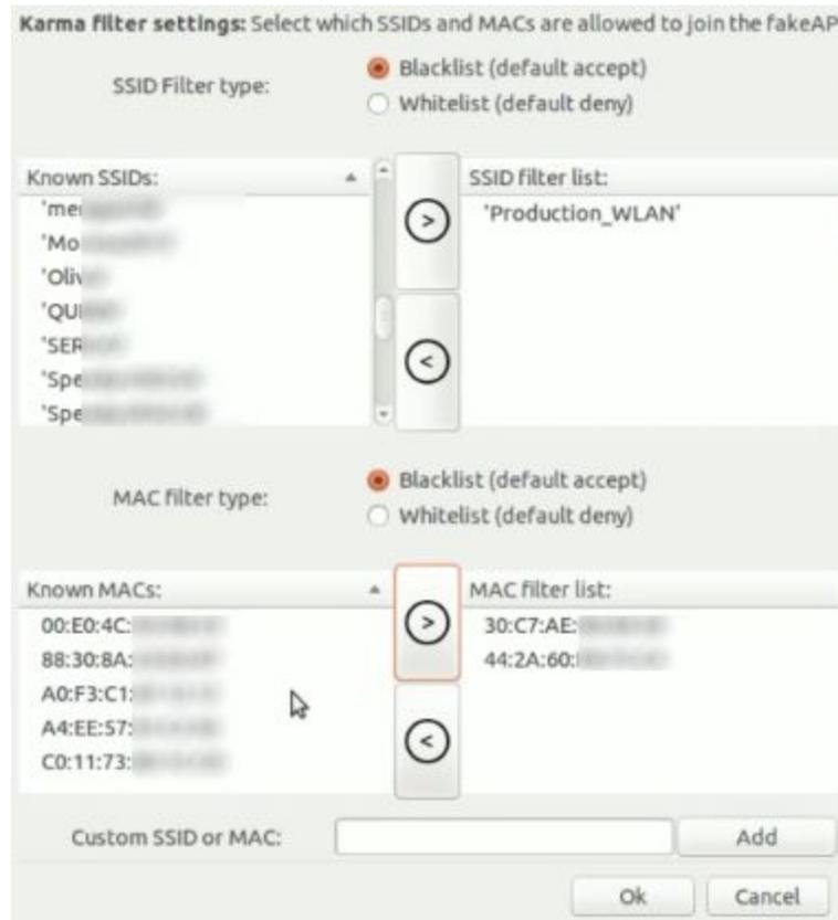
*Karma filter settings dialog. With these settings, any SSID except “Production\_WLAN” will be spoofed, and any station except the two specified MACs will be able to connect.*
